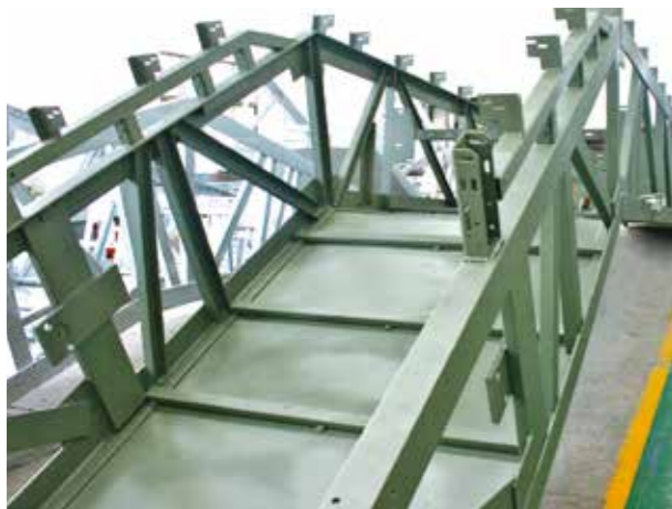
Truss/Painted Angle Steel
